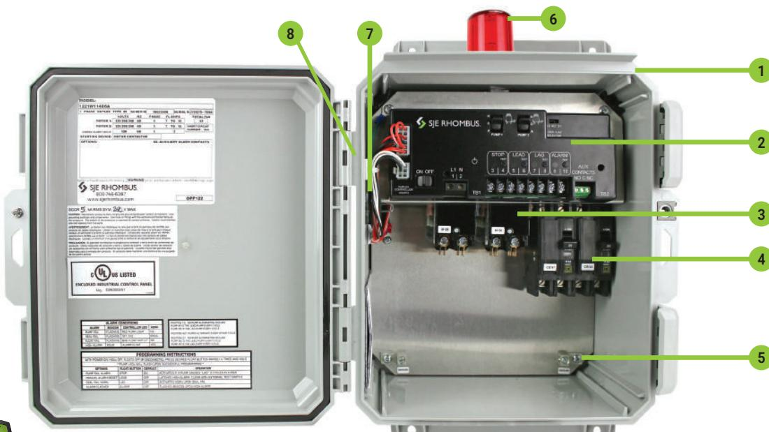
The newly redesigned Model 122 control panel controls two 120/208/240V single phase pumps in water and sewage installations. This panel includes a new innovative duplex controller for pump control, alternation and alarm; including float status LEDs, control/alarm power on/off switch with LED indicator, pump run LEDs, HOA switches, pump lead lag selector switch, auxiliary contacts and more!
