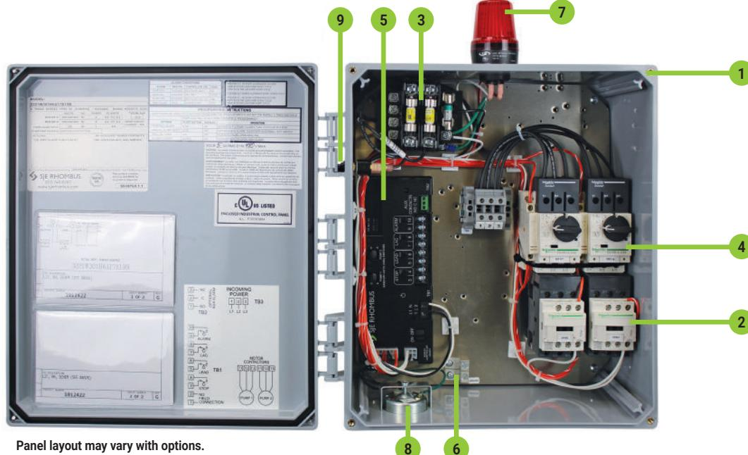
The newly redesigned Model 322 control panel controls two 208/240/480V three phase pumps in water and sewage installations. This panel includes a new innovative duplex controller for pump control, alternation and alarm; including float status LEDs, control/alarm power on/off switch with LED indicator, pump run LEDs, HOA switches, pump lead lag selector switch, auxiliary contacts and more!
