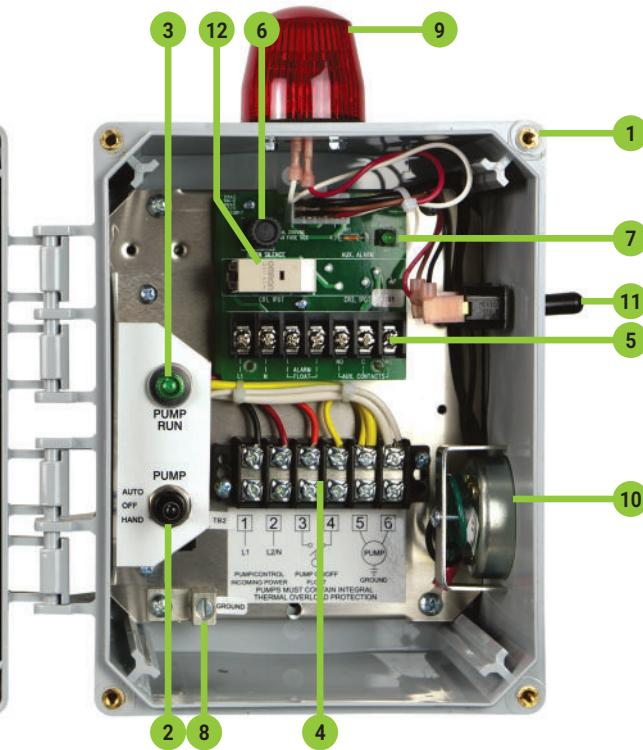
The Model 115 control panel provides customers with a reliable means of controlling one 120, 208, or 240 VAC single phase pump in water and wastewater installations. A pump float switch turns the pump on and off. If an alarm condition occurs, an additional alarm switch activates the audio/visual alarm system. Common applications include pump chambers, sump pump basins, irrigation systems, and lift stations.
