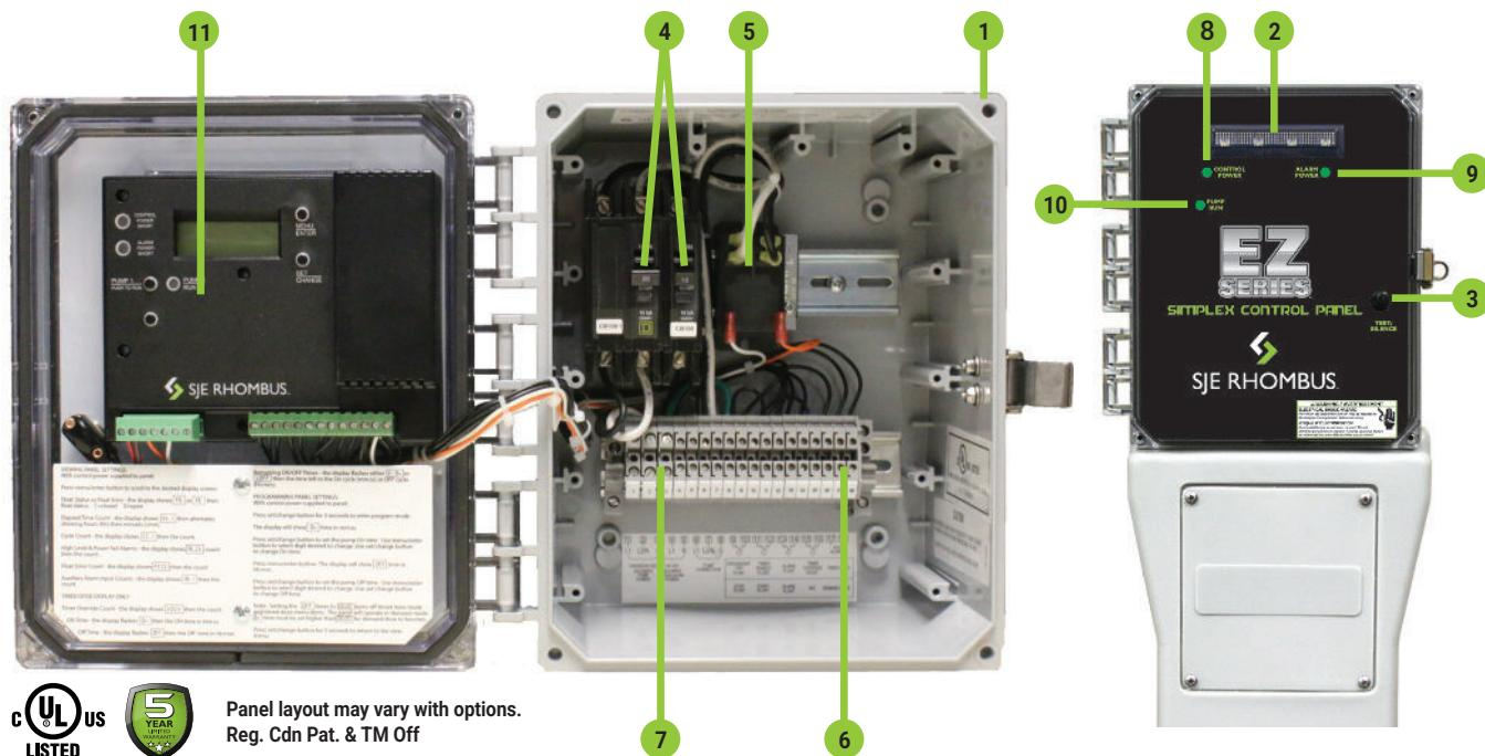
The EZ Series® simplex control panel is designed to control one 120, 208, 240 VAC single phase pump in water and sewage installations.
