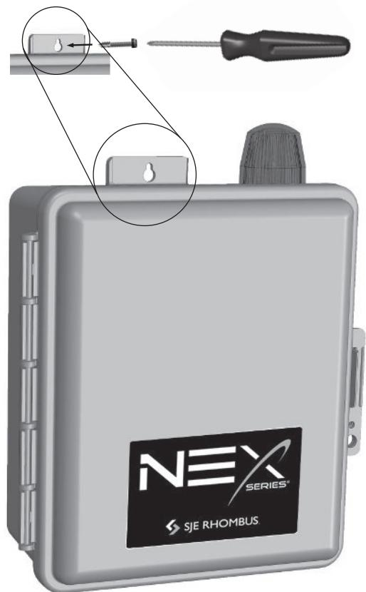
2 Install bottom fastener(s) using appropriate anchors.
