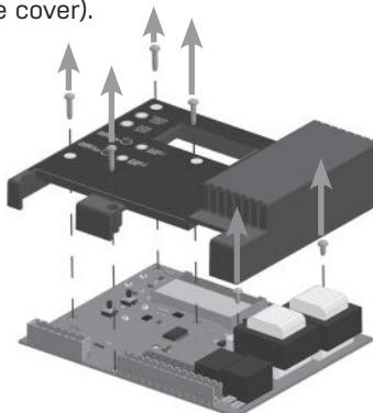
6. Install the new PCA to the panel door with the 2 short 3/8" screws as shown.
