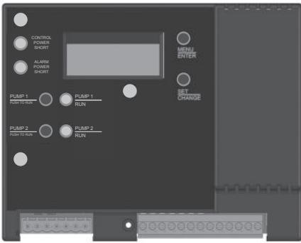
2. Remove molex quick connectors from the circuit board.
