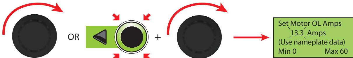
5. Press the rotary selector to save the edited value and exit the editing screen. Or press the ESC button (escape) to exit the editing screen without saving.
