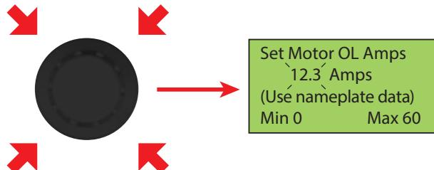
4. Rotate the selector to begin editing the value. Pressing the left arrow button will move the editing position left one digit. This is useful when making large adjustments to the edited value quickly.
