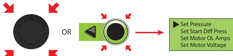
2. Rotate the rotary selector until the selection arrow highlights "Set Motor OL Amps".
