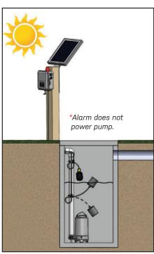
Must be installed in location with adequate sunlight for solar charging. Unit in full alarm without any solar charging will run for approximately 24 hours.
