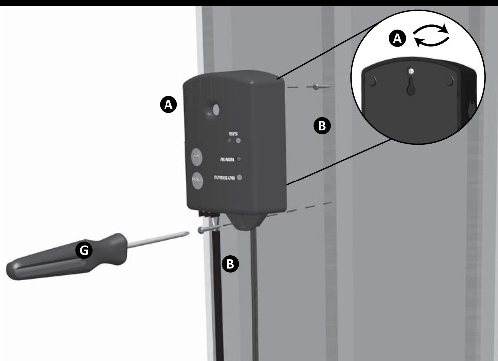
**4** Connect float switch, install battery, and secure power cord to wall outlet.
