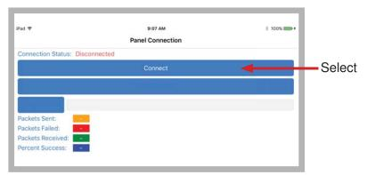
The application displays all available panels that can be connected. The panel name is printed on the label located on the black inner panel. Select the panel name to connect.
