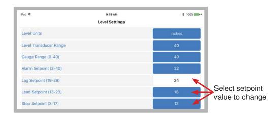
Values shown in parentheses display the minimum and maximum values for the range that can be entered. Minimums and maximums are based on adjacent setpoint values. Setpoint value ranges must meet the following guidelines:
