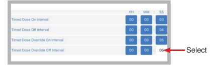
To change the time interval, select the value. A keypad allows a new time to be entered. The time is displayed as HH:MM:SS where HH is hours (0 to 99), MM is minutes (0 to 59), and SS is seconds (0 to 59). The colons do not need to be entered. Select DONE when the correct interval value is entered.
